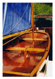
in that the centreboard case was open, and when rowing you sat right on the case and so tended to quickly get a very wet and rather embarrassing rear end. After a couple of outings my Dad quickly made up a suitable plug for the top of the case, which effectively solved that problem.
