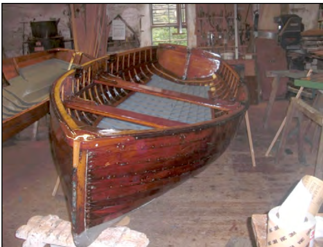
Bow repaired and varnishing begun
