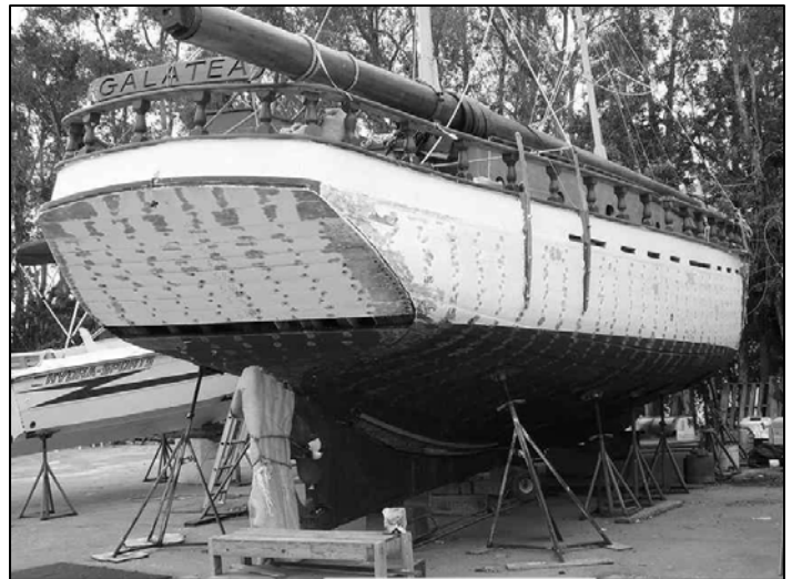
Galatea in the boat yard. At this point in the restoration process she has had several thousand fasteners replaced—as indicated by the “dots”.
